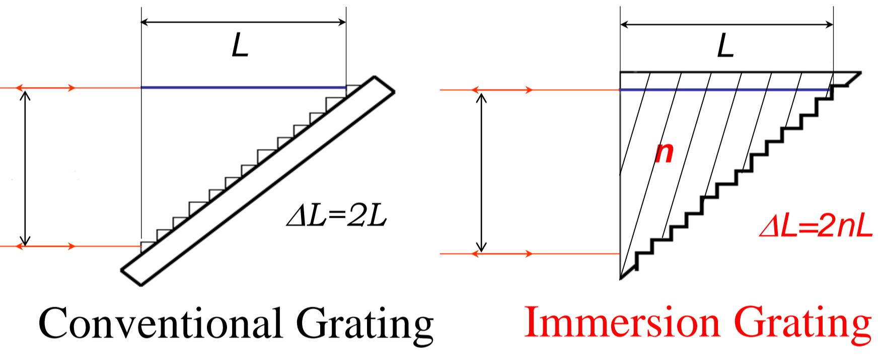
*This study: First fabrication of Germanium ( $n=4.0$ ) Immersion Grating by RIKEN’s ELID (ELectrolytic In process Dressing) Micro-machining Method (Ebizuka et al., 2003).*
