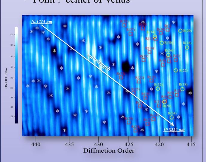
>Echellegram of Venusian atmosphere at 10.1~10.8 μm \*:  ${}^{12}\text{CO}_2 \ v_3 \leftarrow v_1 \ \square$ :  ${}^{12}\text{CO}_2 \ (v_3 + v_2) \leftarrow (v_1 + v_2)$  $\bigcirc$ : <sup>13</sup>CO<sub>2</sub>  $v_3 \leftarrow v_1$
