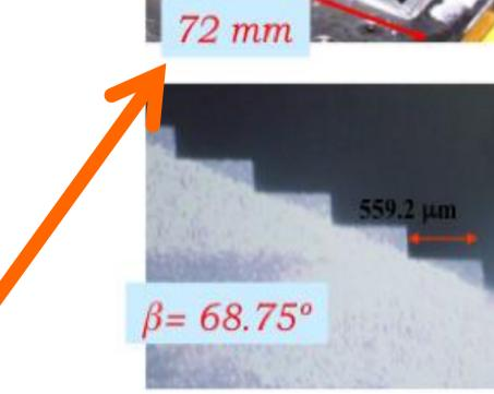
Surface Roughness:11.5 nm rms decrease of *R* by wavefront error: 73 % => real R~38,000
