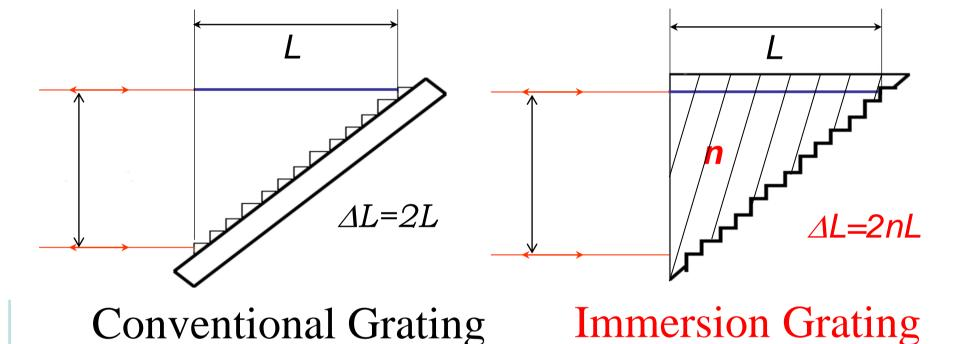
This study: First fabrication of Germanium (n=4.0)Immersion Grating by RIKEN's ELID (ELectrolytic In process Dressing) Micro-machining Method (Ebizuka et al., 2003).
