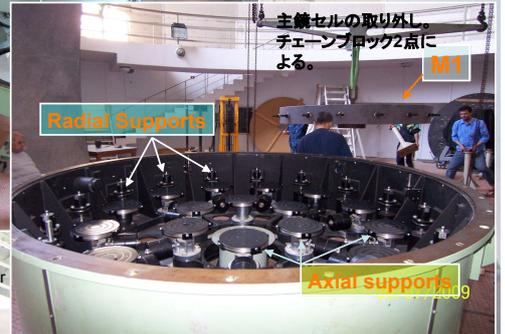
Removing the M1 and its mirror cell. Now the mirror support systems are clearly seen.
