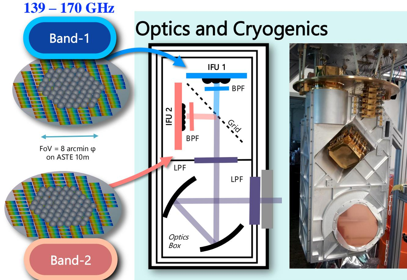
The total number of detectors (voxels) including both Band-1 and 2 will reach ~20,000. The maximum data rate shall be ~100 MB/sec (128 bit, 160 Hz sampling).
