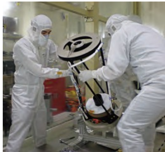
Optical alignment of the telescope
