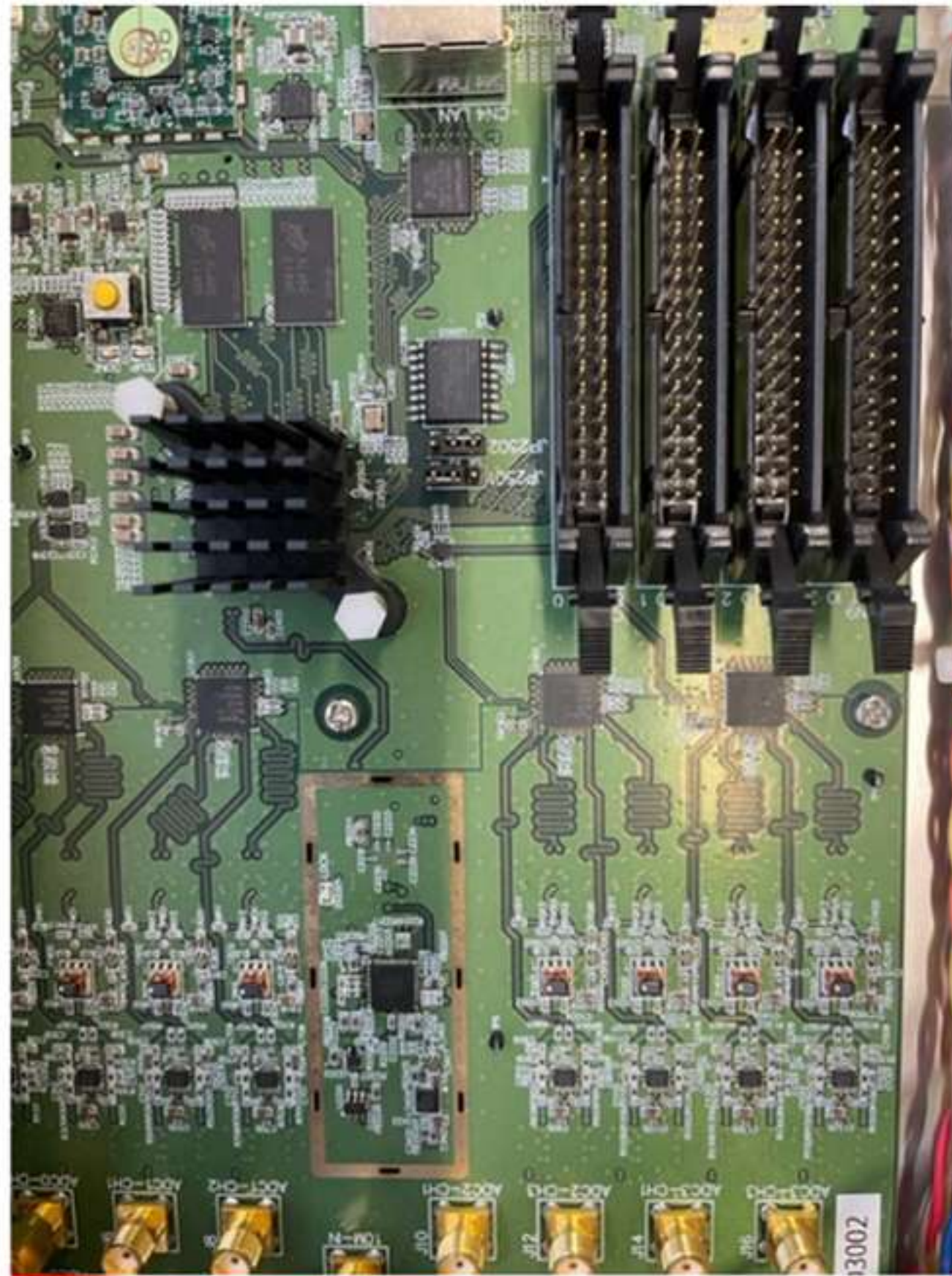
FPGA board for roundtrip phase measurement for 8 stations
