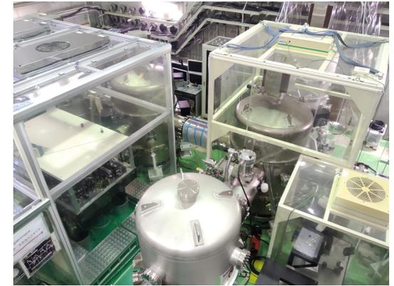
The NAOJ GWSP demonstrated the FDS at 100Hz range **the first in the world.** This technique has been already introduced in Virgo/LIGO.
