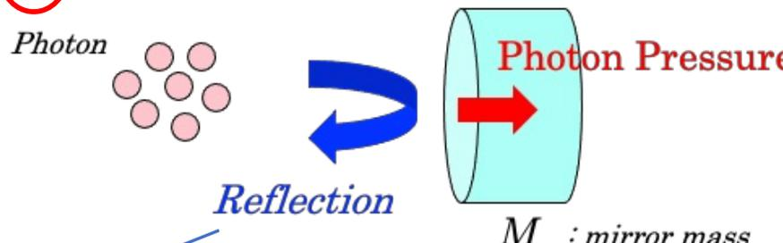
Combination of FDS and heavy mirror is critical to reduce “quantum noise”.
