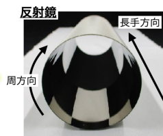
High-precision X-ray grazing incidence mirror
