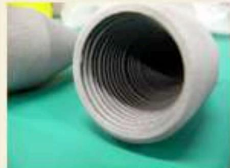
35-50 GHz AlSi10Mg corrugated horn successfully fabricated and tested at cryogenic temperature
