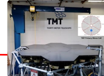
Prototype of the primary mirror cell
