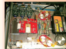
Distribute frequency and time signals with atomic clock precision over a wide area. ⇒ Contribution to 6G ultra-high-speed communication
