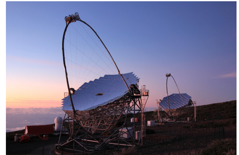
MAGIC-II Stereo System 17m diameter Cherenkov Telescopes
