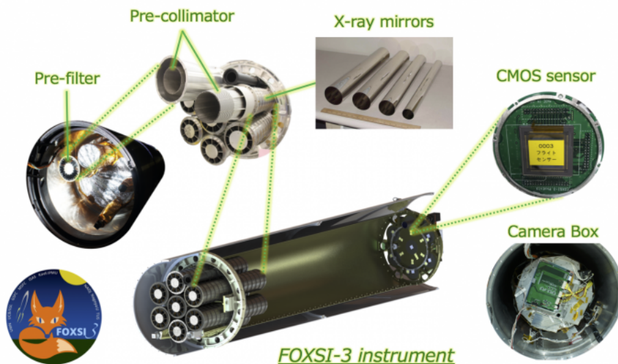
Figure 3. FOXSI-3 soft X-ray instrument. The details of the instrument are described in https://hinode.nao.ac.jp/en/news/topics/foxi-3-180907/ . (© FOXSI-3 team)
