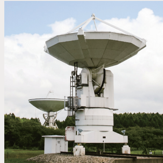
Figure 12: Unit F of the millimeter wave interferometry array at Nobeyama Radio Observatory used by the Radio Astronomy Laboratory of Osaka Prefecture University. The millimeter wave array had used six 10-meter aperture parabolic antennas, but after the end of operation, only Unit F was refurbished for stand-alone use and continued to be utilized. The Nobeyama 45-m Radio Telescope can be seen in the background.
