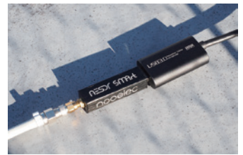
Figure 10: The coaxial cable extending from the dipole antenna was connected to the SDR dongle which in turn was connected to the USB repeater running through a window into our room downstairs. In some cases, noise from a PC can affect the SDR dongle; thus, the SDR dongle sometimes works better when spaced by a hub or repeater than when connected directly to the PC's USB port.
