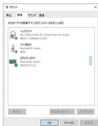
Figure 14: The stereo mixer needs to be enabled to transmit sounds from SDRSharp to MROFFT inside a PC.
