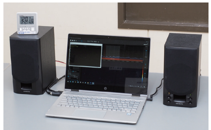
Figure 12: To listen for meteors, external speakers were set up and connected to the PC's headphone jack. When a meteor appears, these speakers give off a short or long echo to let us know its appearance.
