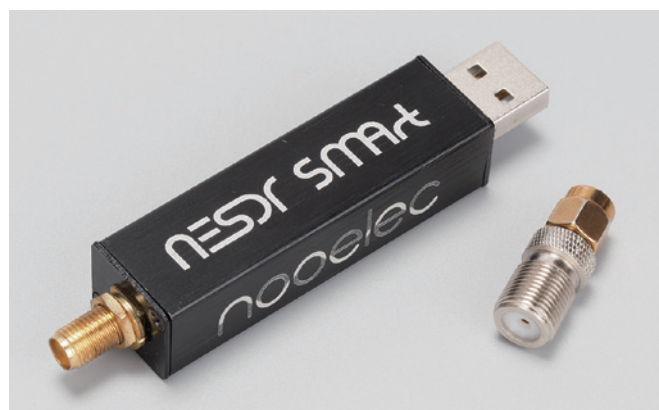
Figure 06: Our SDR dongle of choice was the NESDR SMARt v4 SDR produced by Nooelec, which we purchased online for about 4,000 yen. Among the various types of SDR available, the products we recommend are ones equipped with temperature compensated crystal oscillators (TCXO), which can suppress the fluctuation of the receiving frequency caused by changing temperatures. Because our SDR dongle had an SMA antenna connector (male) and our antenna used an F-type connector (female), we also purchased a conversion adapter (for approximately 400 yen).
