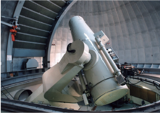
Figure 26: With a 105-cm aperture and 330-cm focal length, Kiso Observatory's Schmidt telescope is the world's fourth largest of its kind and offers a particularly bright field of view. This telescope can now work in a fully remote setting and has been conducting automated observations with Tomo-e Gozen.
