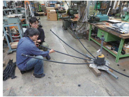
03 The outer ends of the radially arranged pipes were pulled with steel wires toward the center, and these pipes were curved to form an approximate parabolic surface. A stay was inserted into the pipe fitting attached to the middle of each pipe to reinforce the structure. To fix each stay, holes were drilled into the pipe and the fitting, which were then bolted and tightened together.
