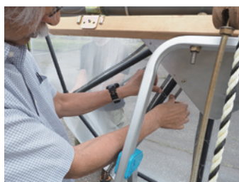
01 First, we prepared the mirror surface. All the team members worked together to attach the metallic mesh.
