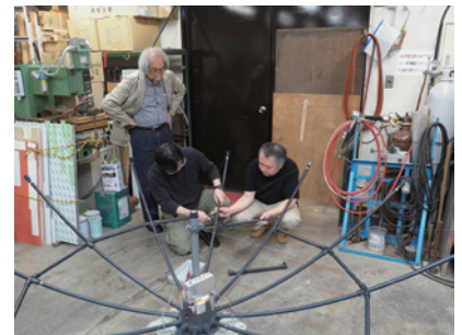
04 The dish frame started to take shape. But one problem arose here: we found that the completed frame would not be able to pass through the workshop door. Anyway, we decided to complete the frame and then disassemble part of it to carry it out of the workshop.
