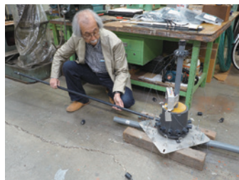
02 The central element of the parabolic antenna is based on an aluminum plate onto which a plastic flowerpot is placed upside down. The steel pipe under the aluminum plate serves as the rotation axis, enabling adjustment of the elevation angle of the antenna. We fixed pipe fittings for PVC pipes around the circumference of the flowerpot and inserted one end of each of the PVC pipes constituting the dish frame into these fittings. By this point, we have already realized that the dish diameter is not 4 m but 3 m.
