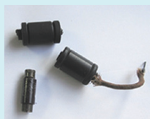
03 Crystal detectors used by Koichi Shimoda in radio observations of the May 9, 1948 solar eclipse.
