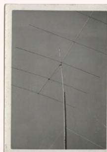
03 (Left) A 6 element Yagi-Uda antenna for 15 m wavelengths (constructed August 1962); (Right) A 2 element loop antenna for 15 m wavelengths (constructed October 1962); after a typhoon struck, I had to construct a new antenna after only two months.
