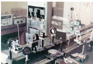
Figure 08: The 128 channel prototype for the first acousto-optical radiospectrometer in the world for cosmic radio waves (1976). It was used for observations on the 6-m millimeter-wave radio telescope and became the model for the Nobeyama 45-m Radio Telescope's large-scale radio spectrometer.
