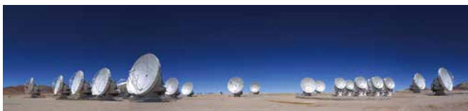
Figure 14: With 66 antennas having diameters of 12 m or 7 m, ALMA, of which Japan is a member, has the world's best performance among radio interferometers observing at millimeter and submillimeter wavelengths.
