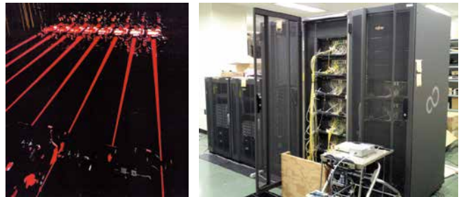
Figure 10: (Left) The large acousto-optical radiospectrometer (AOS) for the Nobeyama 45-m Radio Telescope. 32,000 channels, maximum bandwidth 2 GHz. For 30 years after the start of observations, it yielded many discoveries as the largest radiospectrometer in the world. (Right) the new digital spectrometer now in use, SAM45.
