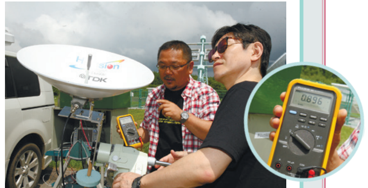
Figures 08 & 09) Then the value went up to a maximum of "0.869 volts" when pointing at the Sun. We've caught radio waves from the Sun.
