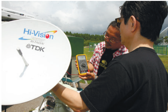
Figure 07) First we measured while pointing at spots far from the Sun. At this time, the tester's readout was "0.598 volts."
