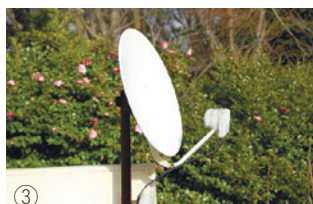
Figure 04) Various familiar receiver antennas. ① is an FM radio extendable/collapsible antenna (rod antenna). ② is a Yagi antenna for ground-based digital TV broadcasts. ③ is a parabolic antenna for BS signals. The receiver and converter are located at the tip of the arm.
