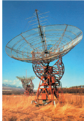
Figure 1) A picture of the 70-600 MHz Radiospectrograph at Nobeyama Radio Observatory used to observe the Sun until 1994. It observed long wavelength radio waves, so it used a metallic mesh parabolic antenna surface. The blue sky in the background shows through it. Unlike the Milky Way's dark stripe, this mirror allows visible light to pass through it and reflects long wavelengths (radio waves).
