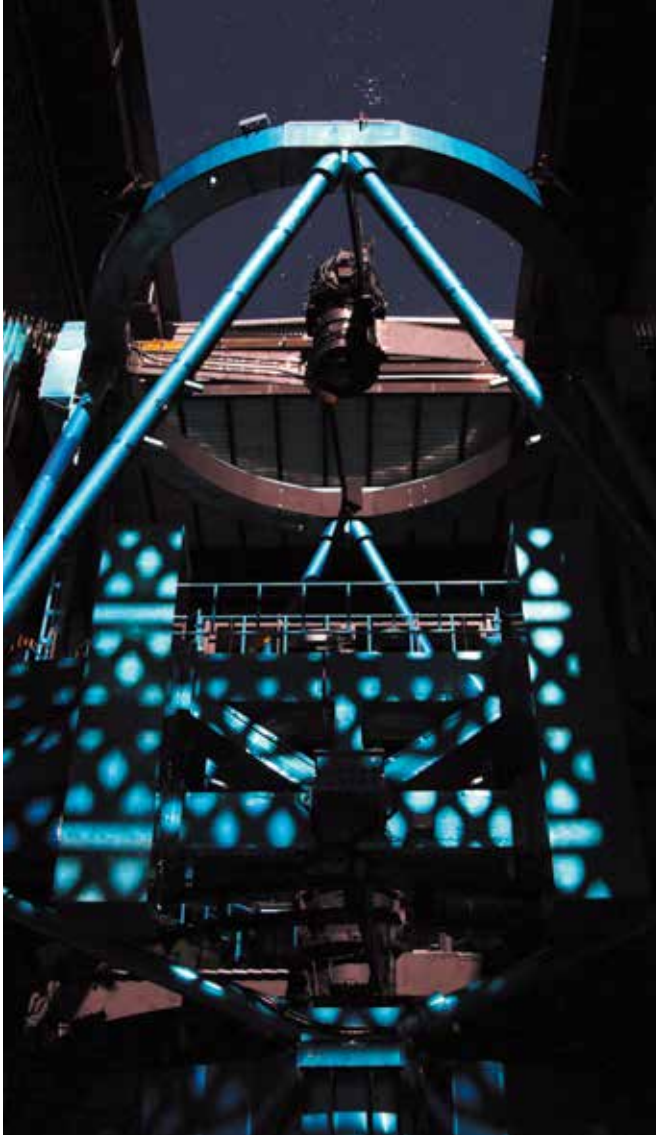
The Subaru Telescope illuminated by moonlight. The ultra-wide field-of-view camera Hyper Suprime-Cam (HSC), is mounted at the top of the telescope structure (prime focus). By attaching a camera at the prime focus with a field of view exceeding one square degree, it is possible to capture an area nine times the size of the full moon in each exposure.
