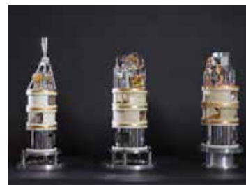
ALMA receivers developed at NAOJ. From left to right: Band 4 (millimeter wave, 125~163 GHz), Band 8 (submillimeter wave, 385~500 GHz), Band 10 (terahertz, 787~950 GHz).
