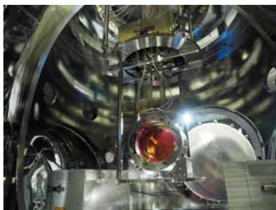
▲The first large suspension system installed into a KAGRA vacuum chamber.
