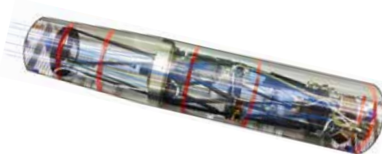
▲ The CLASP instrument for a rocket-borne experiment (to aim for observing magnetic fields in the chromosphere to the transition region in the far ultraviolet range). A similar technique is to be used for the SOLAR-C spectro-polarimetry.
