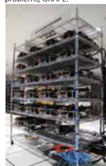
▼ Special-purpose computers for gravitational many-body problems, GRAPE.
