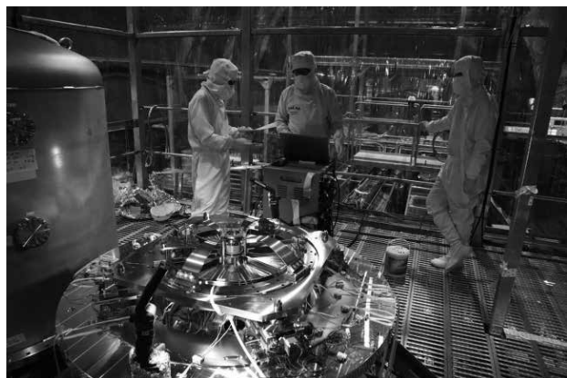
Figure 1: Adjusting the Vibration Isolation System.
