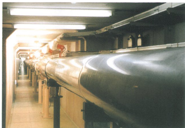
Fig.1 One of the two 300 m vacuum pipes installed in the tunnel. Laser beams travel back and forth inside of them.
