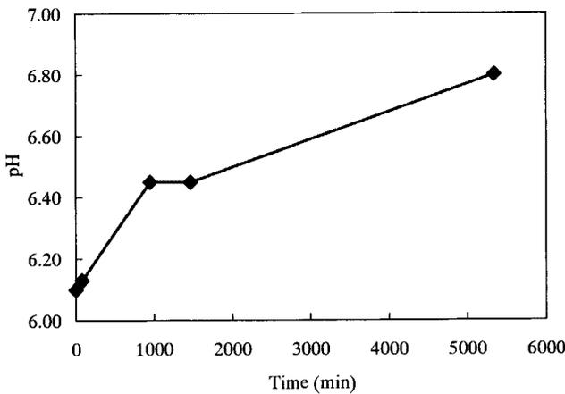
Fig. 3. Relationship between pH value and the time on intact rock sampled from No. 2 site.
