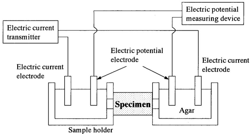
Fig. 4. Layout of the devices for measuring the rock resistivity.
