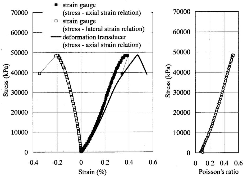
Fig. 6. Stress-axial strain relationship, the stress-horizontal strain relationship and the stress-Poisson's ratio relationship.
