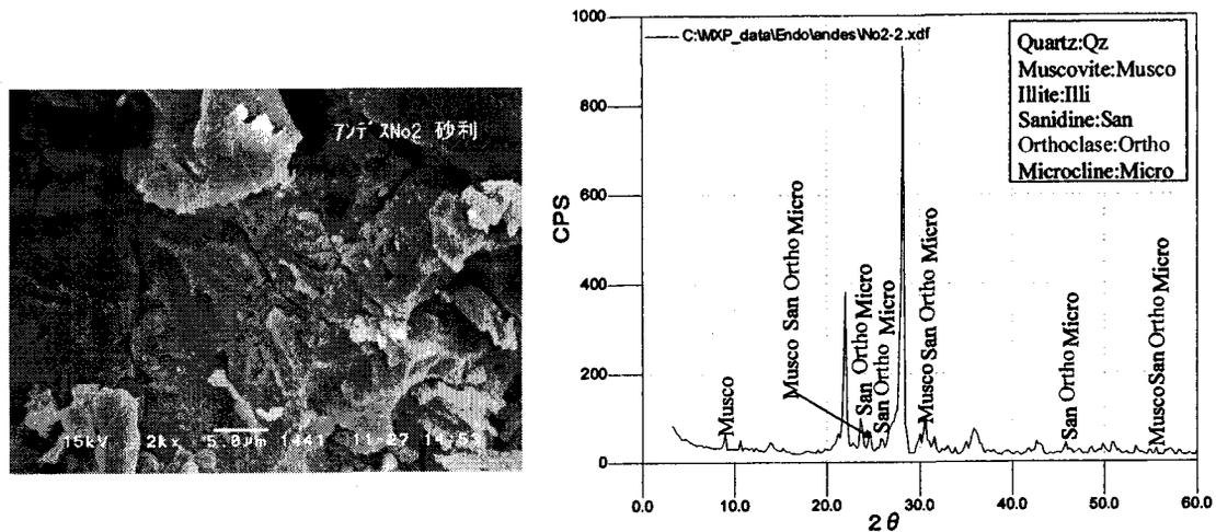
Fig. 2(c). SEM photograph and result by the X-ray diffractometer on sand sampled at No. 2 site.
