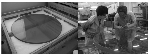
Figure 3: Polishing and measuring processes of mirror segments in Japan. In April 2021, the quality review was conducted for mirror segments that underwent the aspherical polishing process. A total of 13 segments passed the review, which will be followed by the next step of the process, hexagonal shaping.
