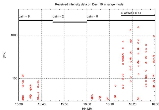
**Figure 2:** Intensity of the received pulses by LIDAR [1]. Experimental conditions of receiver gain (“high” = 8, “low” = 2) and the pointing offset of the ground telescope (el offset = 6 as) are drawn at the top. It is obvious that the reception level changes according to the changes of the observational conditions.
