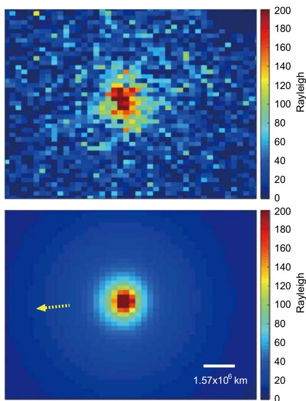
**Figure 1:** Trimmed reduce Ly $\alpha$  (upper) and reproduced (lower) images of hydrogen coma of comet 67P by 2D axi-symmetric model in Rayleigh units on UT 2015 Sept 13. Yellow arrow is solar direction.
