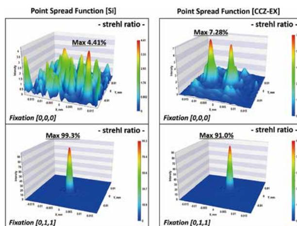
**Figure 2:** Strehl ratios of the aberrated focus image by CCM. [Upper left] CCM made of Si fixed on 3 points perfectly. [Lower left] CCM made of Si fixed on 3 points and one of them is perfectly. [Upper right] CCM made of CCZ-EX<sup>®</sup> fixed on 3 points perfectly. [Lower right] CCM made of CCZ-EX<sup>®</sup> fixed on 3 points and one of them is perfectly.
