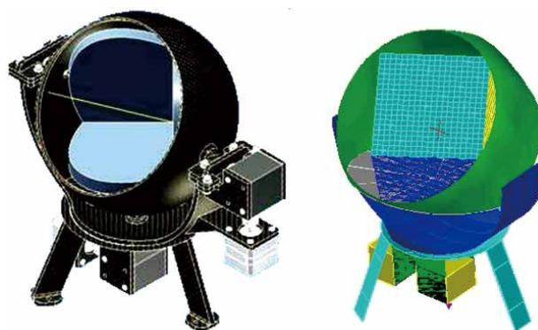
**Figure 1:** [left] General view of the CCM system. [right] Mathematical model of the CCM system for Thermal Desktop<sup>®</sup>. CCM aperture is 20 cm.
