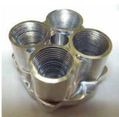
Figure 1: A broadband corrugated horn array [1].
