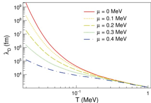
**Figure 1:** The Debye length for the  $^3\text{He}+^7\text{Be}$  reaction as a function of temperature (in MeV) for several electron chemical potential assumptions.
