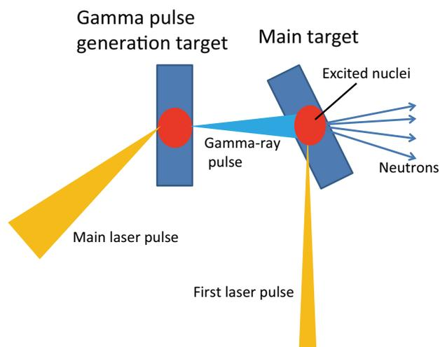
Figure 1: Schematic view of experiment.
