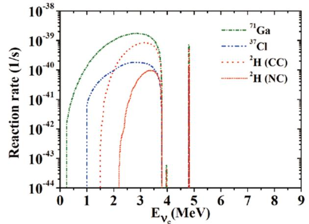
Figure 2: Reaction rates via  $^{37}\text{Cl}(\nu_e, e^-)^{37}\text{Ar}$ ,  $^{71}\text{Ga}(\nu_e, e^-)^{71}\text{Ge}$ ,  $^2\text{H}(\nu_e, e^-pp)$  and  $^2\text{H}(\nu_e, \nu_e np)$  reactions. The neutrinos are generated from decay of  $^{27}\text{Si}$  which are produced by the 15 MeV and 10 mA proton beam on a  $^{27}\text{Al}$  target.
