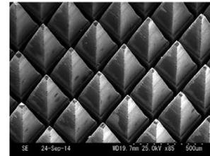
Figure 2: Broadband anti-reflective structure for Silicon [2].
