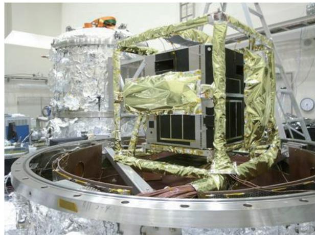
**Figure 2:** Nano-JASMINE STM at the NAOJ space chamber just before the thermal vacuum test. Test heaters which control outer temperature are equipped around STM.
