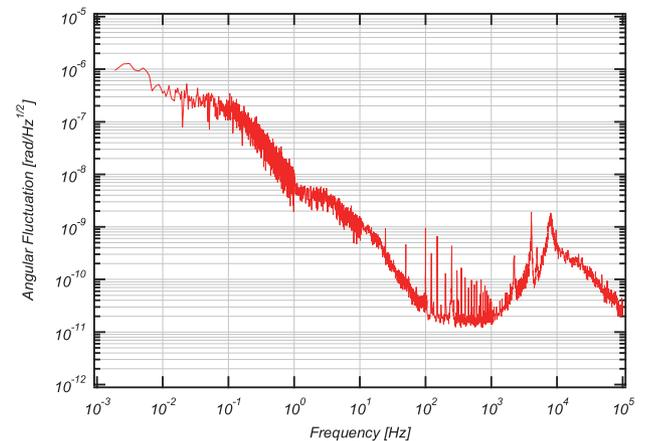
**Figure2:** Power spectral density of the measured differential angle fluctuation of the two mirrors forming Fabry-Perot cavity.
