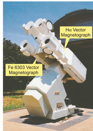
Figure1: The current configuration of the Solar Flare Telescope.
