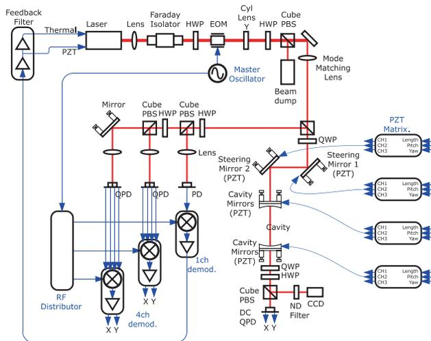
**Figure1:** Schematic diagram of the optical, electronic, and servo-control systems for the basic angle monitor.
