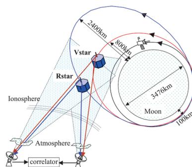
**Figure1:** Concept of the same-beam differential VLBI observation for SELENE project.
