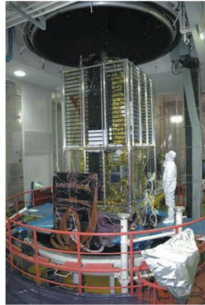
**Figure2:** SOLAR-B spacecraft at the ISAS space chamber just before the thermal vacuum test. The satellite was surrounded by aluminium frames equipped with test heaters to control outer temperatures.
