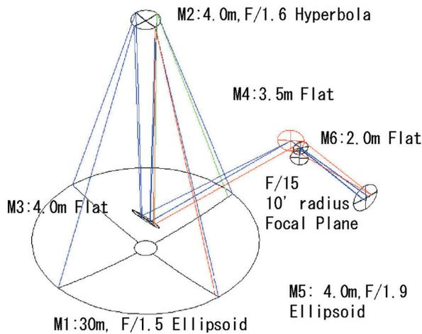
Figure1: Three-Mirror Anastigmat Layout.
