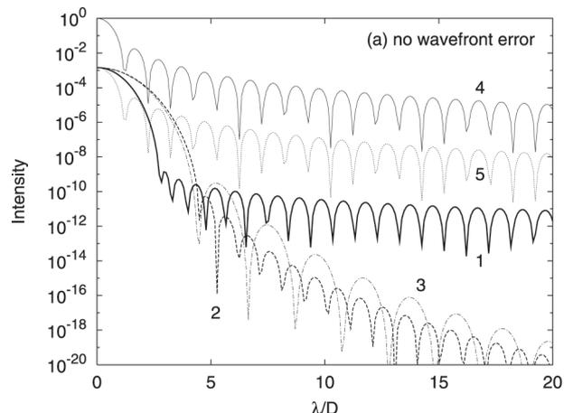
**Figure2:** Intensity profiles along the high-contrast axis for combinations of nulling interferometer with modified pupils. The profiles for three modified pupil under nulling interferometer destructive conditions are shown (1, 2, 3). In the case of the circular aperture we show both constructive condition (4) and destructive nulling condition (5).
