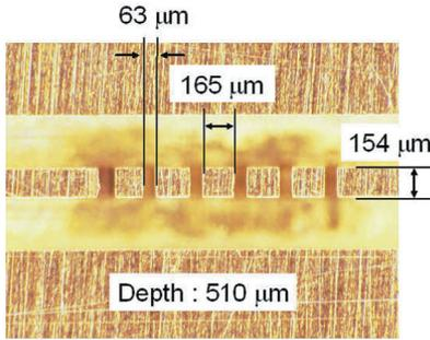
**Figure2:** Results of the mechanical measurements of the RF quadrature hybrid.
