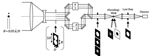
**Figure1:** Coronagraphic optics by pre-optics nulling interferometer combined with modified pupil method.
