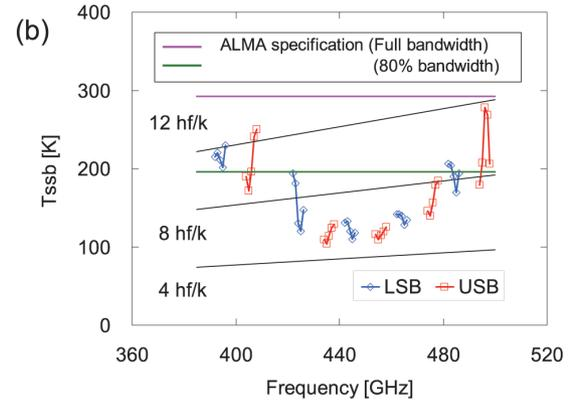
**Figure3:** (a) Image rejection ratio, (b) single-sideband (SSB) noise temperature of the ALMA Band 8 cartridge-type receiver [4] using the 2SB mixer.
