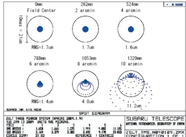
Figure2: Spot diagram with diffraction circles.
