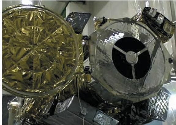
**Figure1:** SOLAR-B spacecraft when the front door of Solar Optical Telescope (SOT) was opened. SOT was located at the center, X-Ray Telescope (XRT) on the lower right, and EUV Imaging Spectrometer (EIS) on the upper left.
