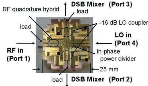
**Figure1:** Photograph of an RF/LO coupler. An RF/LO coupler contains an RF quadrature hybrid, two LO couplers, and an in-phase power divider.
