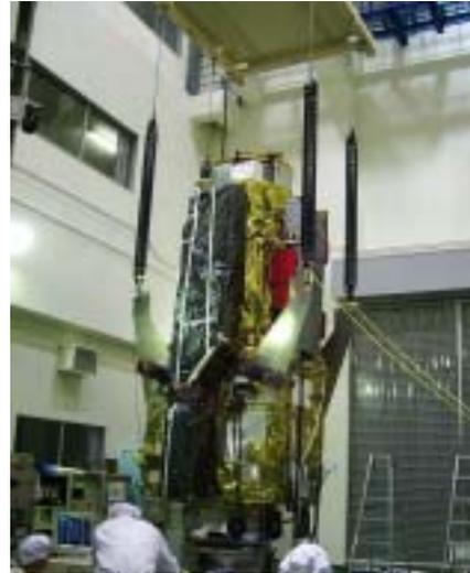
**Figure2:** Micro-vibration test configuration to measure a response of the Optical Telescope Assembly for moving components in the spacecraft that act as sources of disturbance.
