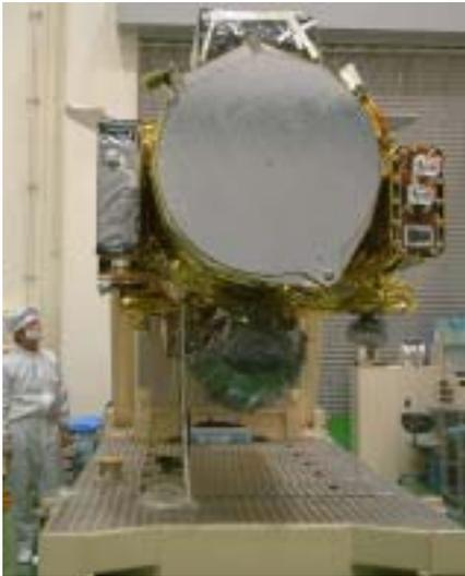
**Figure1:** Telescope apertures of the flight model Solar-B spacecraft. The Optical Telescope Assembly is at the center and its Focal Plane Package is on the left. X-ray Telescope and EUV Imaging Spectrometer on the bottom and top are covered with black baggings for protection from external contamination.
