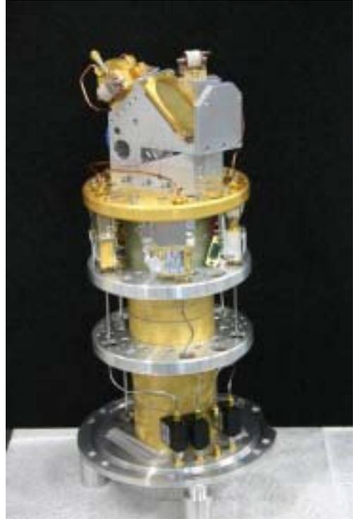
**Figure2:** A photo of ALMA band 8 cartridge Qualification Model.
