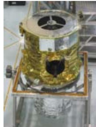
**Figure1:** SOLAR-B Optical Telescope prior to top- and side-door installation in NAOJ clean room.
