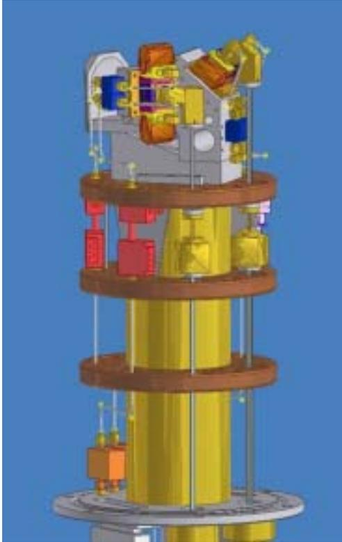
**Figure1:** Design of ALMA band 8 cartridge Qualification Model (QM).
