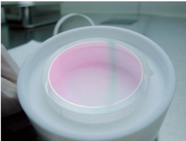
Figure 1: CLU G1 lens with a coating by IBS .
