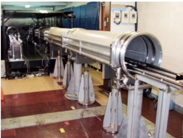
Figure 4 : 8 m vacuum optical delay line .
