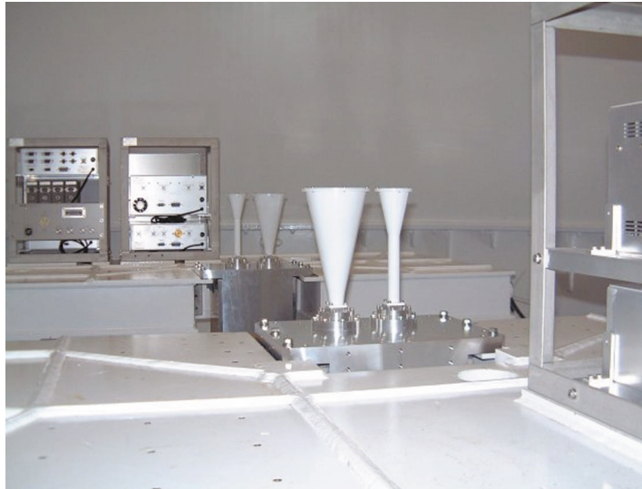
Fig. 3. Dual-beam receivers mounted on the dual-beam platform. Each receiver has two horns for 22 GHz and 43 GHz. Two boxes on the left are local oscillator and electro-optical transformer.
