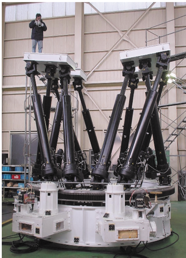
Fig. 2. Dual-beam platform system. Two receivers will be mounted on two platforms that are sustained by six arms.
