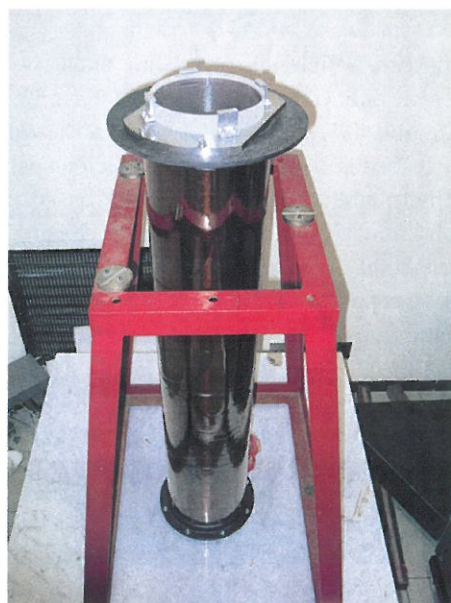
Fig. 2. Thermal model of ILOM telescope.
