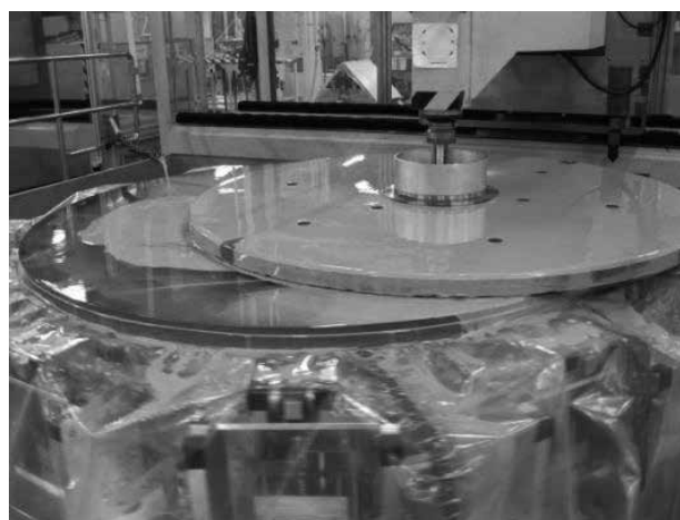
Figure 3: Aspherical grinding of a mirror segment of the primary mirror (provided by Canon).
