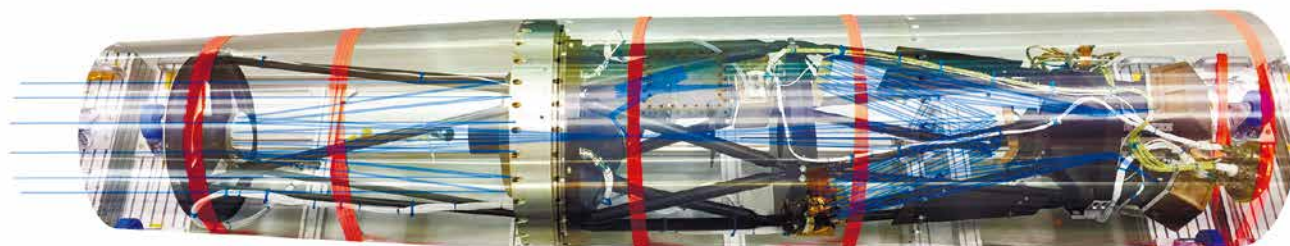
Figure 2: The assembled CLASP instrument. When the CLASP is launched, the instrument is covered with the rocket skin (semitransparent shell in this picture). The optical path is indicated with blue lines.
