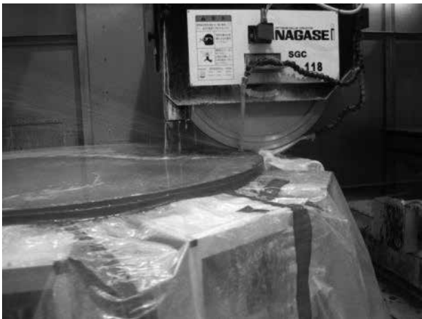
Figure 4: Aspherical grinding of a primary mirror segment.
