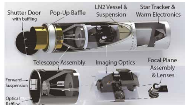
Figure 1: Model of the CIBER-2 instrument. A 28.5 cm Cassegrain telescope directs light into the imaging optics, where beam splitters divide the light into three imaging optics (Arm-S, Arm-M, Arm-L). Each optical path travels to one of three focal plane assemblies, where a broadband filter subdivided the light into two wavelength bands which are both recorded by a single detector array for a total of 6 bands. A small segment of each detector array is also covered by a linear-variable filter. The imaging optics is mounted to an optical bench that connects the Cassegrain telescope assembly to a liquid nitrogen cryostat. Radiative shielding is provided by a radiatively-cooled door and cryogenically-cooled pop-up baffle that extends during observations.
