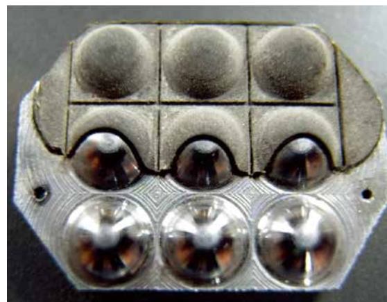
Figure 2: Si lens array and mixed epoxy anti-reflection layer (upper half). Slits reduce thermal stress of the Si and the AR [3].
