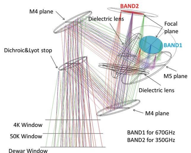
**Figure 2:** Cold optics. The rays reflected by the ellipsoidal mirror go through a cryostat window. The dichroic filter divides incoming rays into two bands. Each ray is focused at the focal plane after a flat mirror and a high density polyethylene lens, and couples with a conical horn.
