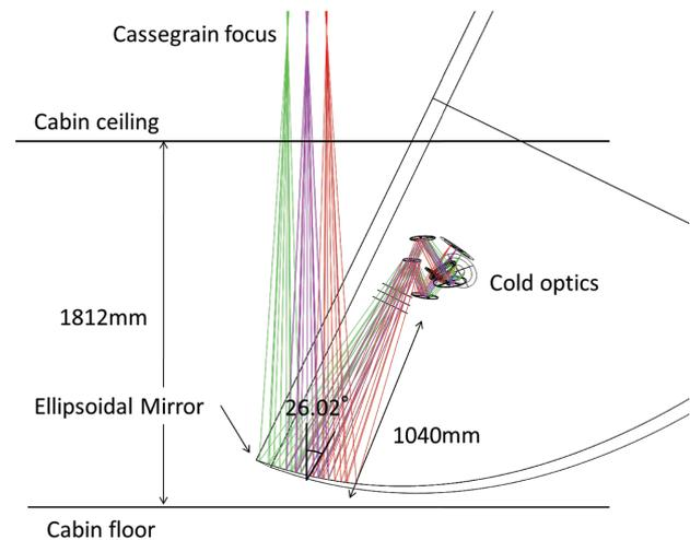
**Figure 1:** Receiver cabin optics. The rays reflected by the main- and sub-reflectors focus near the ceiling of the receiver cabin, and go into the receiver cabin. A modified ellipsoidal mirror optimized by adding fifth-ordered polynomials to reduce aberration is located near the bottom of the cabin to refocus the outspreading rays into the camera cryostat.
