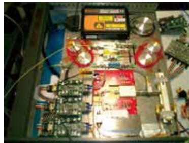
The photonic technique to produce terahertz frequency radio waves from an optical laser.
