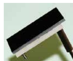
A newly developed megapixel CCD (2048 × 4096 pixels and 30 mm × 60 mm light receiving surface).
