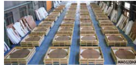
A special glass with an extremely low thermal expansion rate is used for TMT's primary mirror segments, which comprise part of Japan's contribution. As of March 2024, 356 mirror blanks have been produced.
