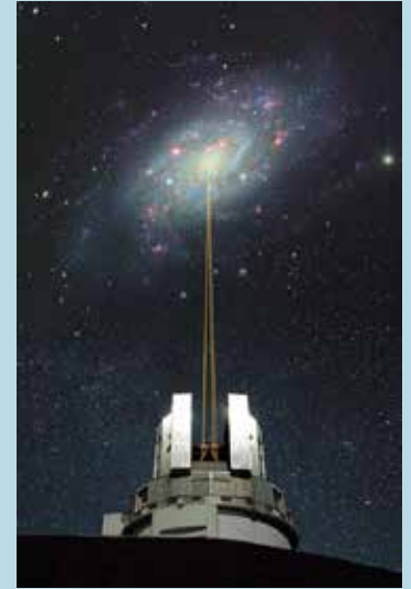
By directing four laser beams into the sky and making the upper atmosphere glow, wide-field adaptive optics create artificial stars (laser guide stars), which enable us to measure and compensate for the blurring by Earth's atmosphere. (Conceptual Image)
