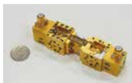
A novel superconducting microwave amplifier made by connecting frequency mixers.
