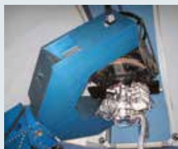
A CCD camera mounted on the telescope for tracking space debris. Credit: JAXA
