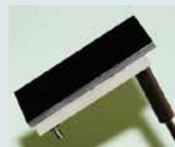
A newly developed megapixel CCD (2048 \times 4096 pixels and 30 mm \times 60 mm light receiving surface).
