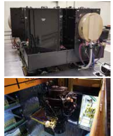
The wide-field multi-object spectrograph, Prime Focus Spectrograph (PFS), is mounted at the prime focus of the Subaru Telescope. It can simultaneously observe up to 2,394 objects across its 1.3 degree diameter field-of-view. (top) One of the spectrograph modules in the telescope dome. (bottom) The Prime Focus Instrument, together with the Wide Field Corrector, mounted at the prime focus of the telescope.
