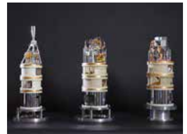
ALMA receivers developed at NAOJ. From left to right: Band 4 (millimeter wave, 125~163 GHz), Band 8 (submillimeter wave, 385~500 GHz), Band 10 (terahertz, 787~950 GHz).
