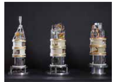
ALMA receivers developed at NAOJ. From left to right: Band 4 (millimeter wave, 125~163 GHz), Band 8 (submillimeter wave, 385~500 GHz), Band 10 (terahertz, 787~950 GHz). Credit: ALMA (ESO/NAOJ/NRAO)
