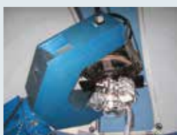
A CCD camera mounted on the telescope for tracking space debris. Credit: JAXA
