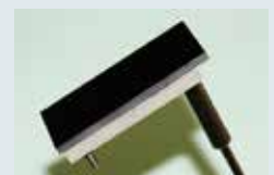
A newly developed megapixel CCD (2048 \times 4096 pixels and 30 mm \times 60 mm light receiving surface).
