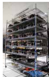
▲Special-purpose computers for gravitational many-body problems, GRAPE.
