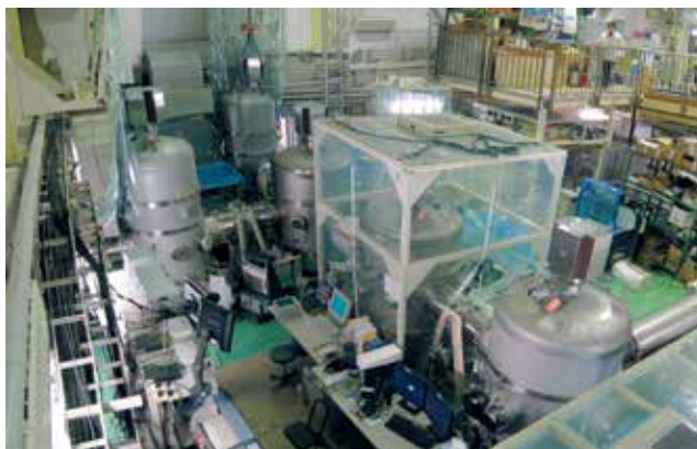
▲Central parts of TAMA300. Main optical components of the laser interferometer are installed in vacuum tanks connected by vacuum tubes.
