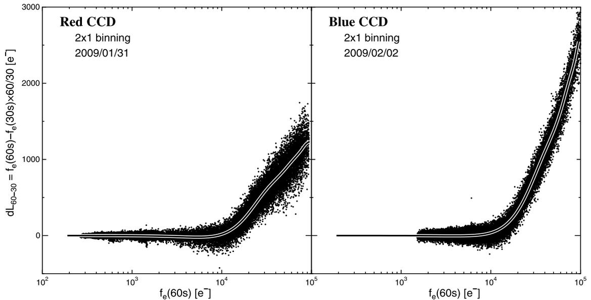
**Fig. 4.** Count difference ( $dL_{60-30}$ ) measured from the apparent counts at exposure times of 60 s and 30 s. The left (right) panel shows the result obtained for the red (blue) CCD in the  $2 \times 1$  (spatial  $\times$  wavelength) binning mode. Solid lines show the fitting results for each measurement point; fitting is performed with ninth-order polynomials. Nonlinearity effects are clearly observed for electron numbers greater than  $10,000e^-$  in both the CCD chips.
