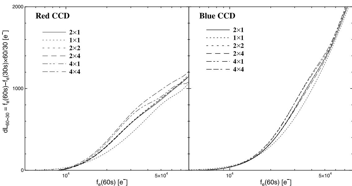
**Fig. 6.** Fitting results for  $dL$ , shown in equation (9). The differences between the results for various binning modes are considerably smaller than the difference between the red and the blue CCD chips. In particular, the curves for  $2 \times 1$ ,  $2 \times 2$ , and  $2 \times 4$  binning are in good agreement for both chips.
