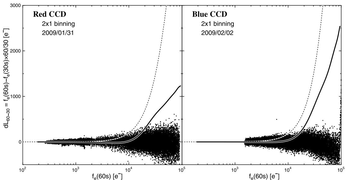
**Fig. 5.** Count difference ( $dL_{60-30}$ ) after our correction. Solid lines are the same as those ones in figure 4. Dotted lines show the correction curves ( $F_{\text{raw}} - F_{\text{cor}}$ ) derived from the fitting curves shown by solid lines. Corrected data show a very flat  $dL$  for all the count, indicating that the correction is valid up to  $100,000e^-$ .
