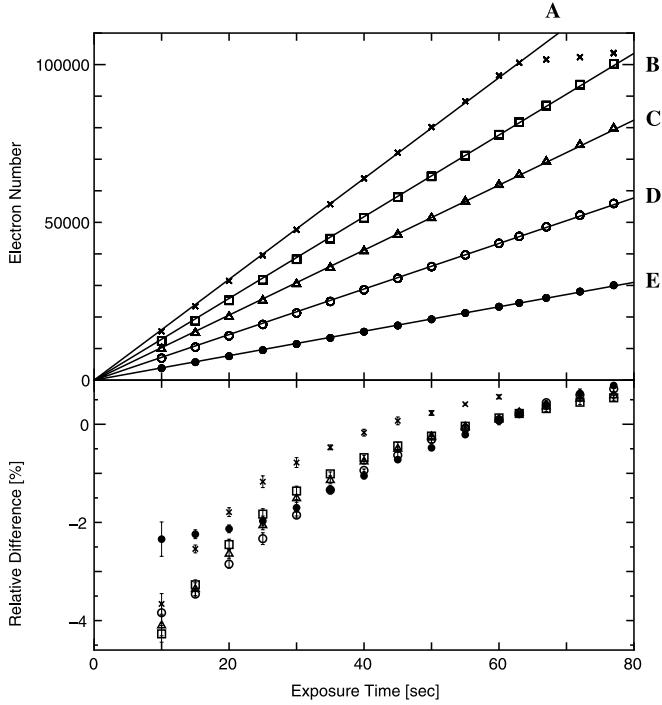
**Fig. 3.** Correlation between signal counts and exposure times. The upper panel shows electron numbers as functions of exposure time for the five regions mentioned in figure 1. The solid lines indicate linear fits to the data points. Saturation effect is observed in Region A when electron number exceeds  $100,000e^-$ . The lower panel shows the departure from the linear fit. Error bars show the standard deviations of the last six of the ten measurements.
