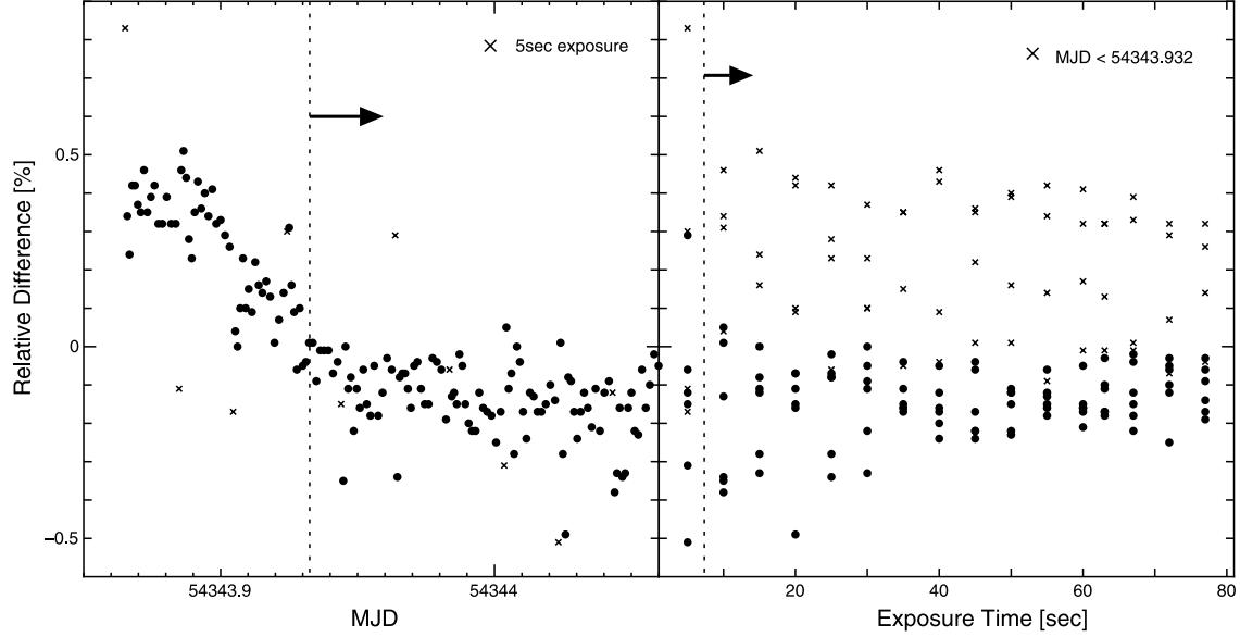
**Fig. 2.** Relative difference among the counts in the flat spectra obtained at different exposure times for investigating the stability of the intensity of the halogen lamp and the shutter opening and shutter closing times. The left panel shows the results as functions of measurement time (MJD: modified Julian date), while the right panel depicts the results as a function of exposure time.
