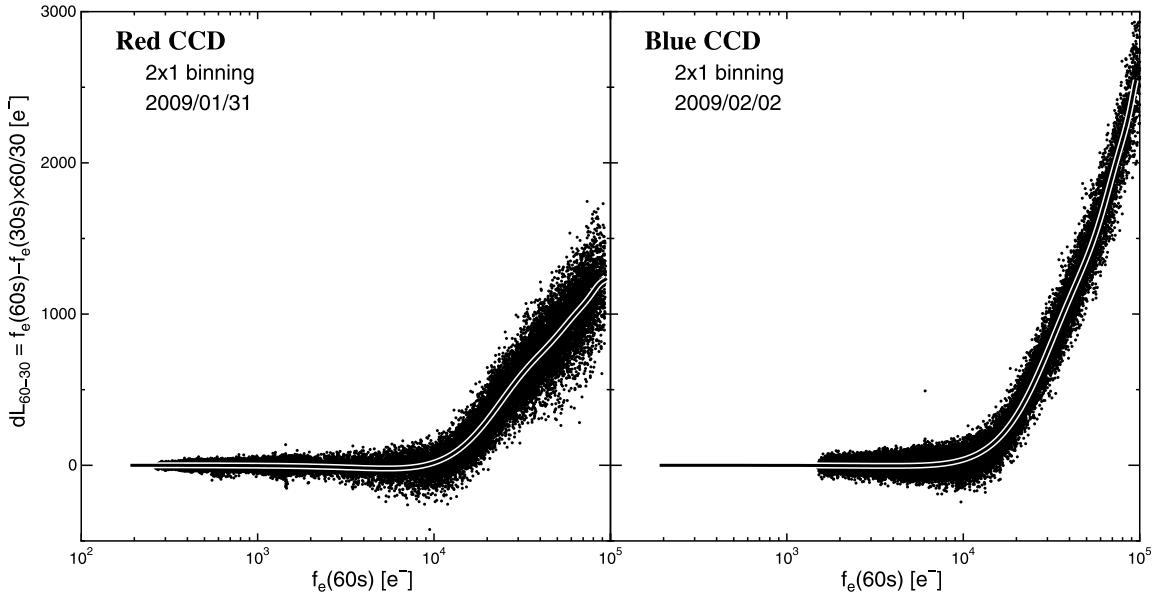
**Fig. 4.** Count difference ( $dL_{60-30}$ ) measured from the apparent counts at exposure times of 60 s and 30 s. The left (right) panel shows the result obtained for the red (blue) CCD in the  $2 \times 1$  (spatial  $\times$  wavelength) binning mode. Solid lines show the fitting results for each measurement point; fitting is performed with ninth-order polynomials. Nonlinearity effects are clearly observed for electron numbers greater than  $10,000e^-$  in both the CCD chips.
