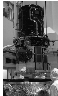
Figure2: Upside-down OTA-FM is being hoisted down to lower part of a vacuum chamber for opto-thermal test (in the clean room of NAOJ).
