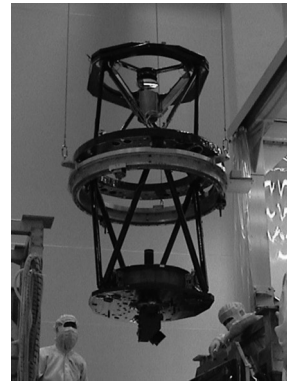
Figure1: OTA-FM is being hoisted out of an integration tower into another support frame for installation of heaters, temperature sensors, cables, and envelopes after the initial optical assembly and test (in the clean room of NAOJ).
