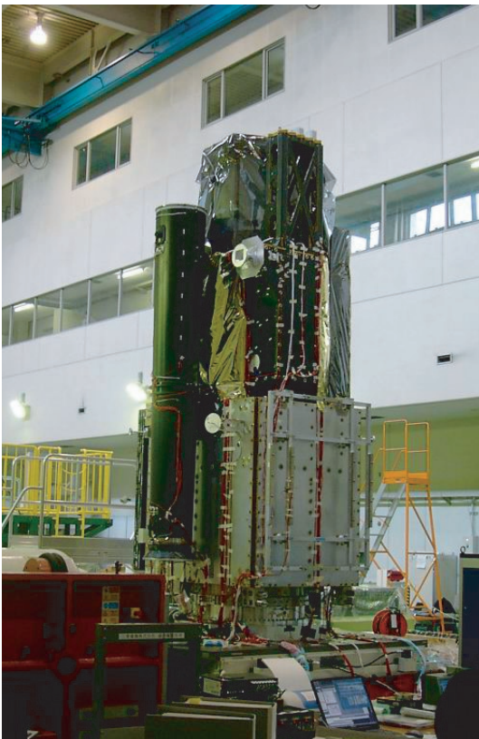
Figure 2: The Solar-B Mechanical Test Model mounted on the ISAS vibration test facility.
