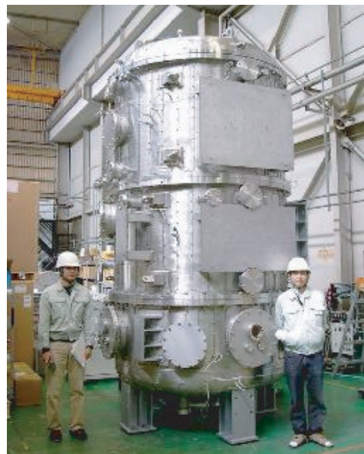
Figure 8: Vacuum chamber for opto-thermal test of OTA.
