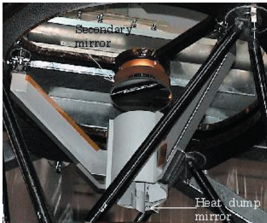
Figure 6: Secondary mirror and heat dump mirror (HDM) of OTA
