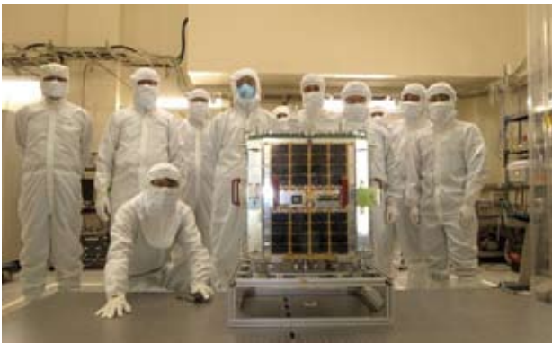
Figure 1: The Nano-JASMINE flight model in the ATC large clean room after experiments of optical alignments.
