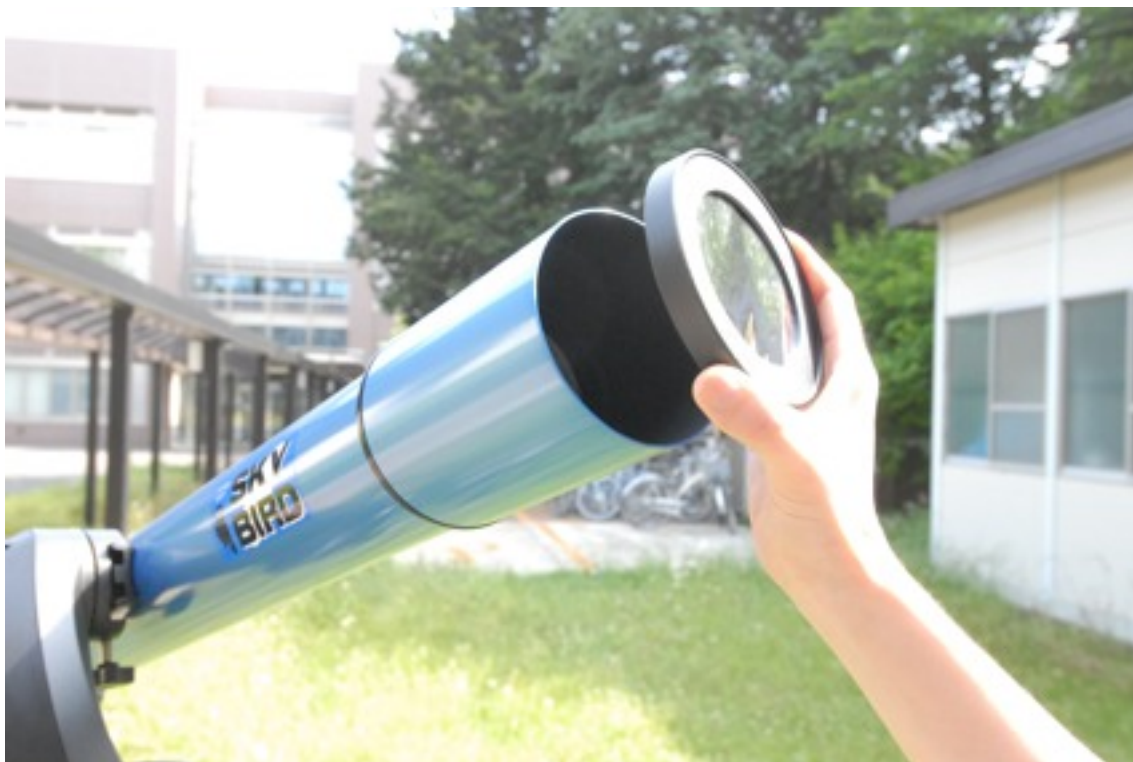
Some models include a special filter in the package. (The model in the photo is Skybird AT-MACS - 80L)
