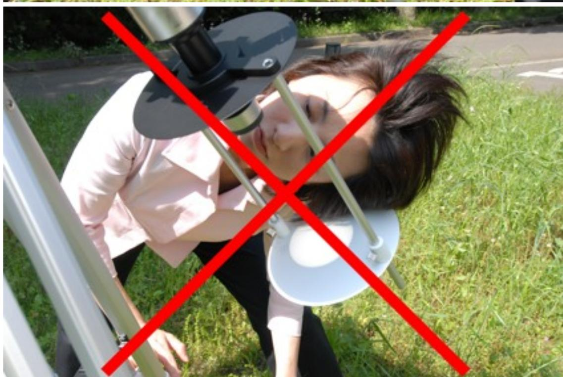
**It is very dangerous to insert body parts into or to look through the path of light.**
