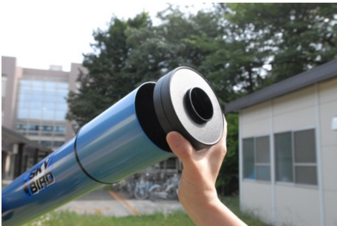
If it is a little too bright when you look through the filter, tightly fix the aperture cap onto the frame of the filter.
