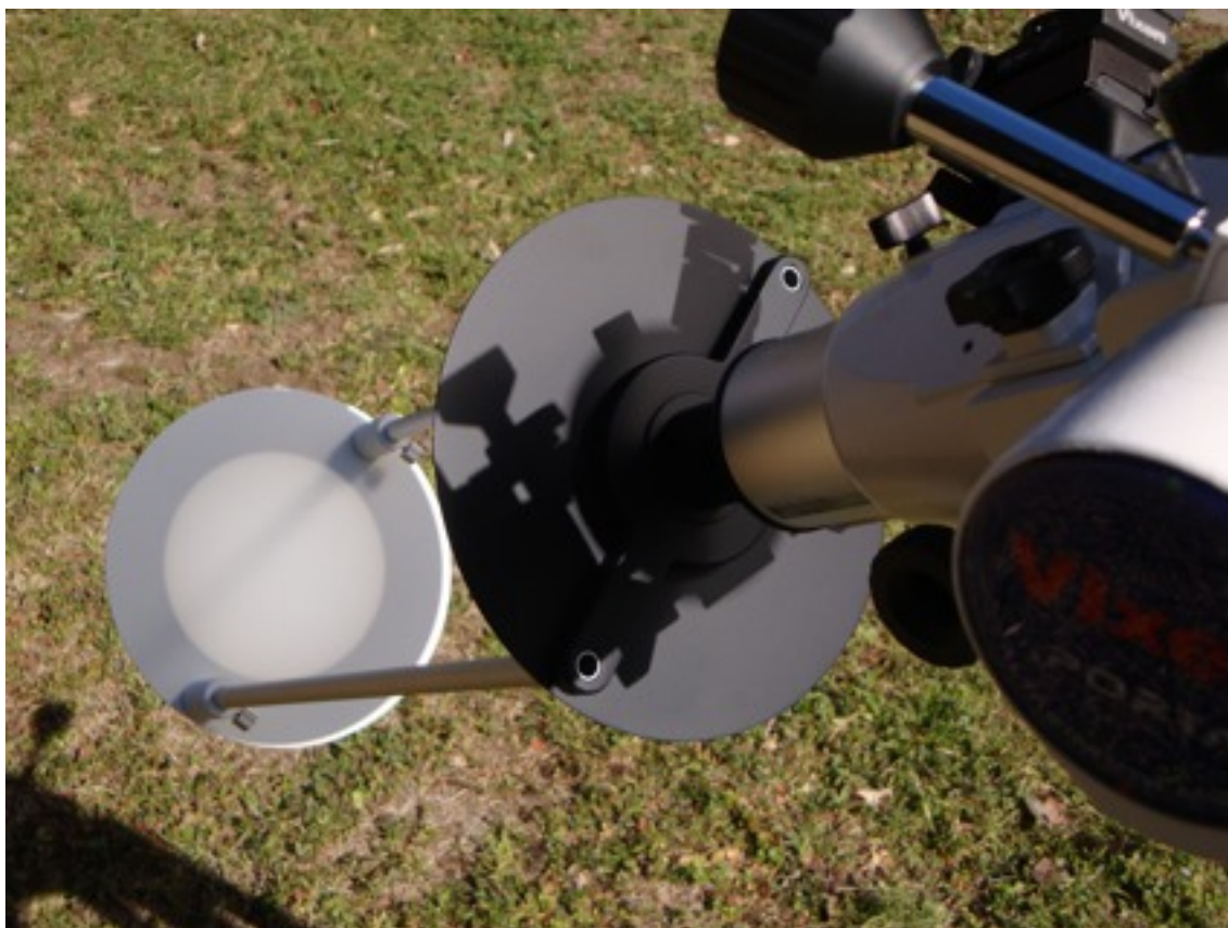
Example of a Solar Projection Screen in use (The model in the photo is Vixen's "Solar Observation Set 2009")
